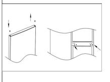
6. Install the bottom hinge to the left side of cabinet, then install two adjustable feet on the current position, then install the freezer door.
