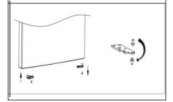
5. Remove the hinge hole cover from right side of freezer door, then install to left side. Remove the center hinge screw cover on the left side of cabinet, then install its to right side of cabinet.
