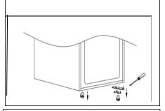
4. Remove the right door stopper on the bottom of fridge and freezer door, then get the left door stopper from the accessory bag, install it on the bottom left side of fridge door and freezer door. Remove the pin shaft and install to other side.
